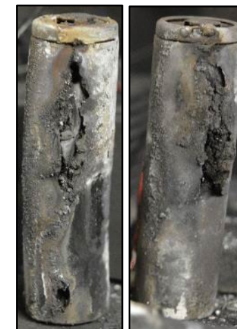
Photos taken of cells following a thermal runaway experiment.
