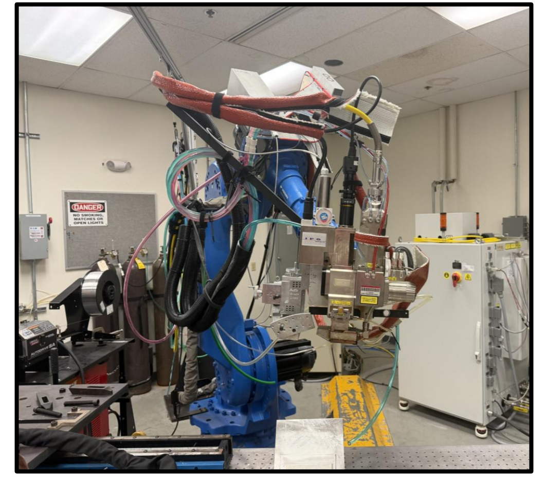
Figure 1. IPG Photonics YLS-6000 fiber laser System used to produce welds; 1070 \mu\text{m} wavelength, 600 \mu\text{m} spot size.
