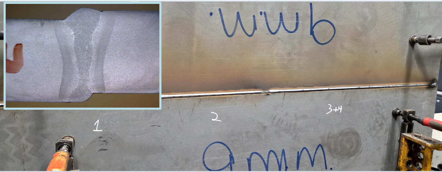
Fig. 1a Robotic HLAW butt weld on the 9 mm × 9 mm Strenx® test plate (plate 56) clamped in the Cloos cell, Haiger, Germany. Zero-gap square groove, single pass, arc-leading; positions 1–4 mark the downstream sectioning locations.
