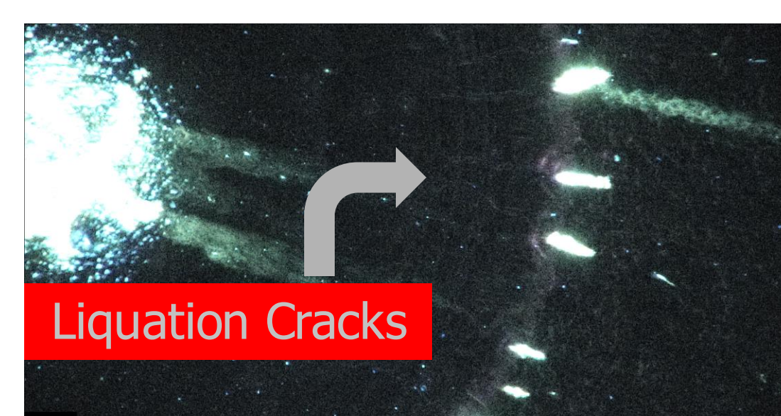
Fig 6. Cu-Ni WADED-T (penetrant without developer)
