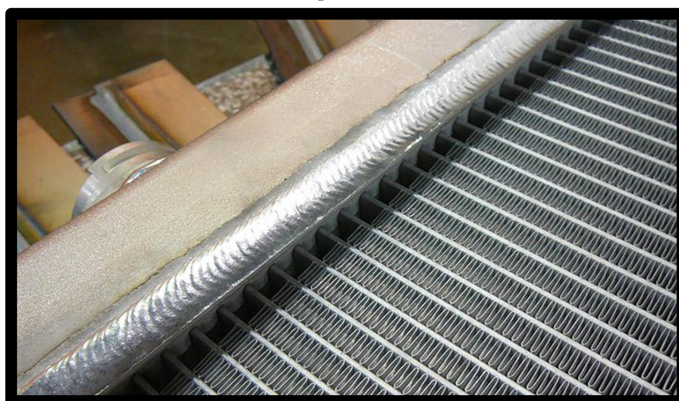
Optimized Weld (Balanced Parameters)
