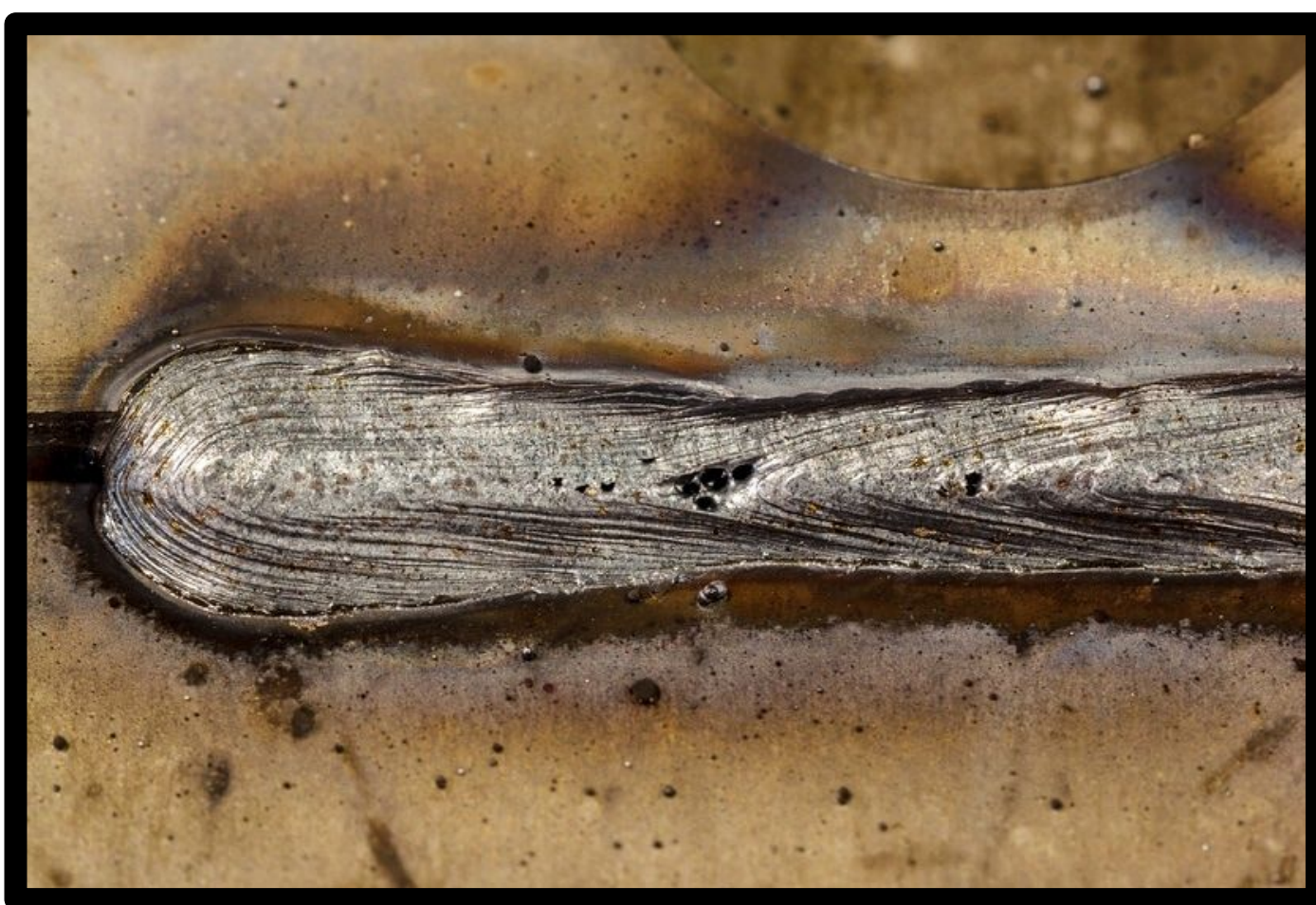
Defective Weld (Improper Parameters)
