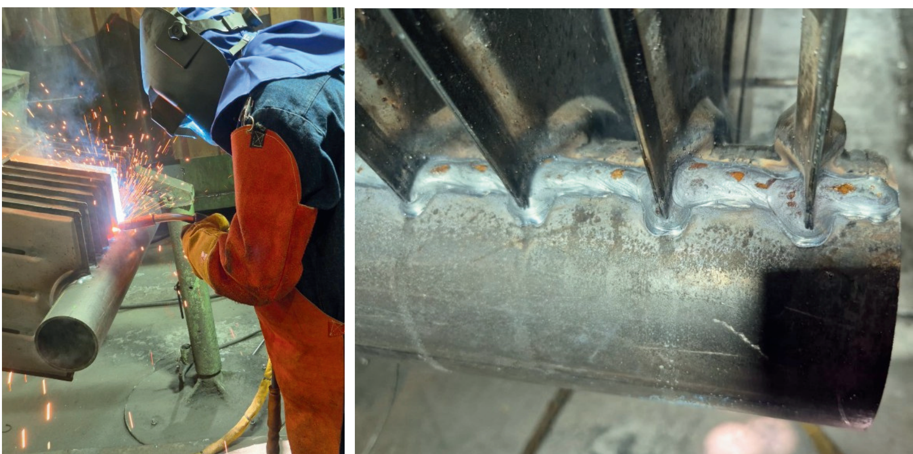
Figure No. 1 GMAW Welding Tube / Steel Sheet Sample Production
