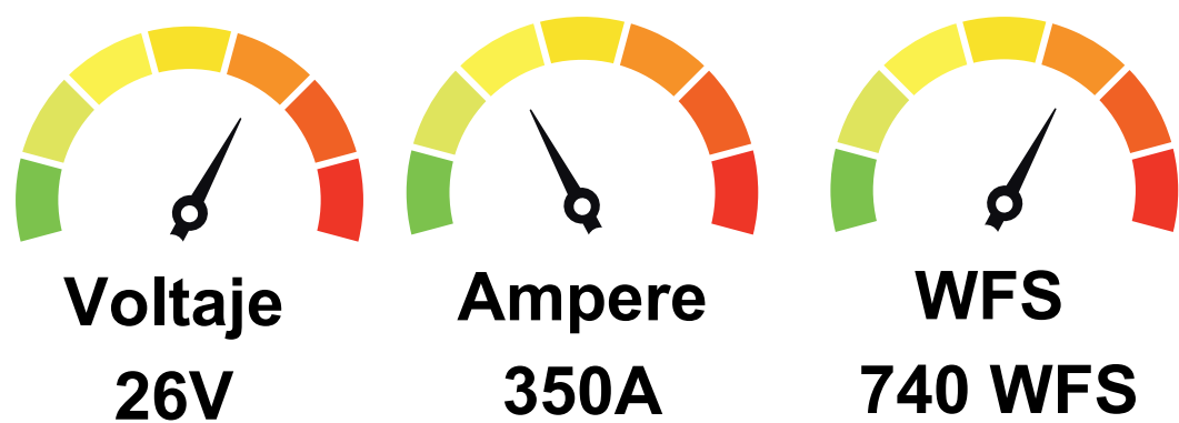
Figure No. 6 Welding Parameters Performance
