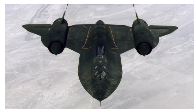
The Blackbird, made of 85% titanium, was one of the fastest spy planes.
