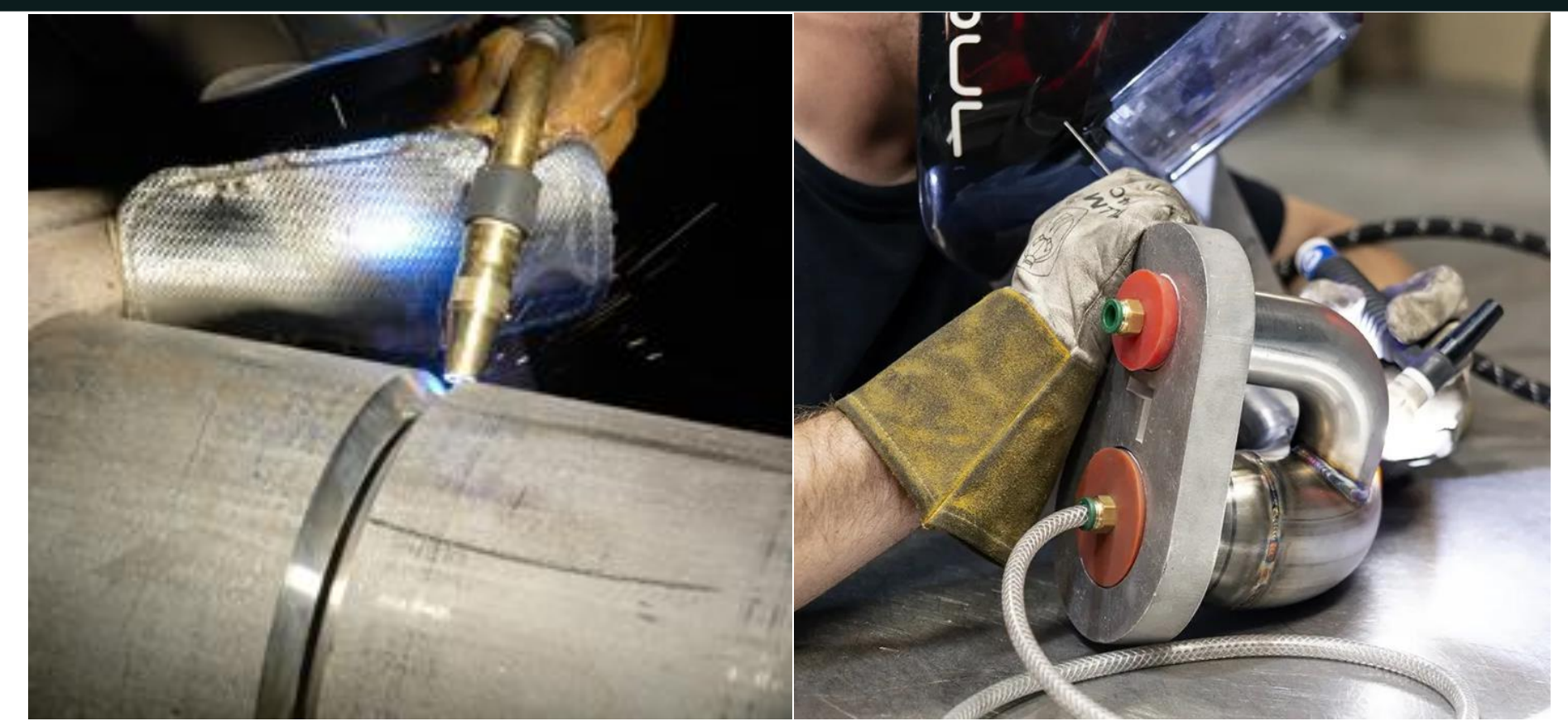
Images of welding stainless steel piping using GMAW and GTAW processes with back purging (Source: Miller Electric)
