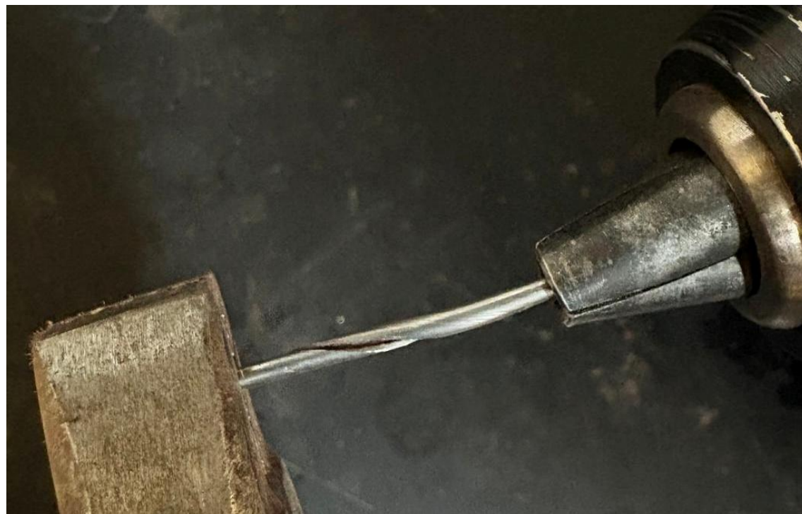
Fig. 3 – Wire sheath opened using pliers and drill rotation
