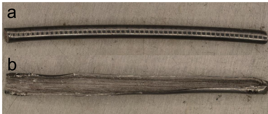
Fig. 4 – Wire sheath (a) before and (b) after flux removal
