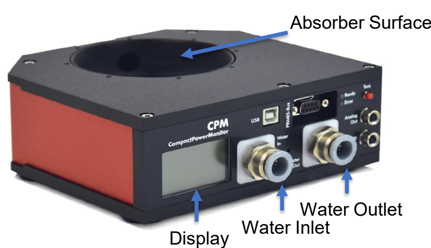
Figure 3: PRIMES Compact Power Monitor used for laser power measurement.
