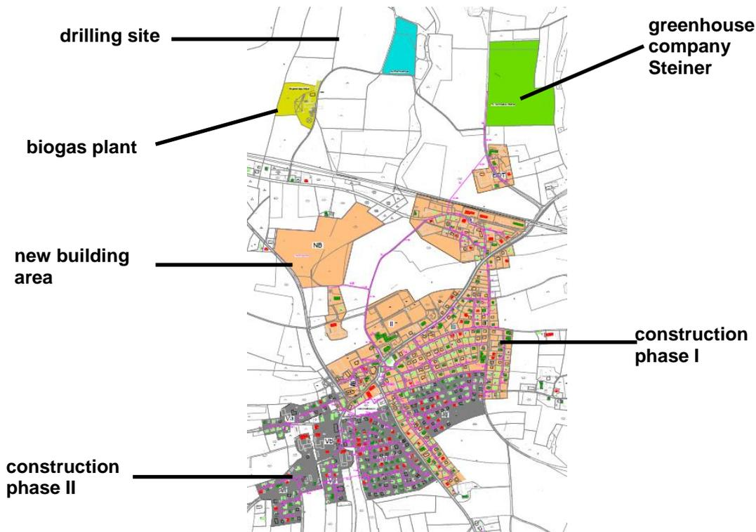
In the picture above, the vegetable gardening company Steiner (green), the drilling site (blue) and the biogas plant of Guido Mayer (yellow) are shown. In addition, the development area and the construction phases I and II can be seen.
