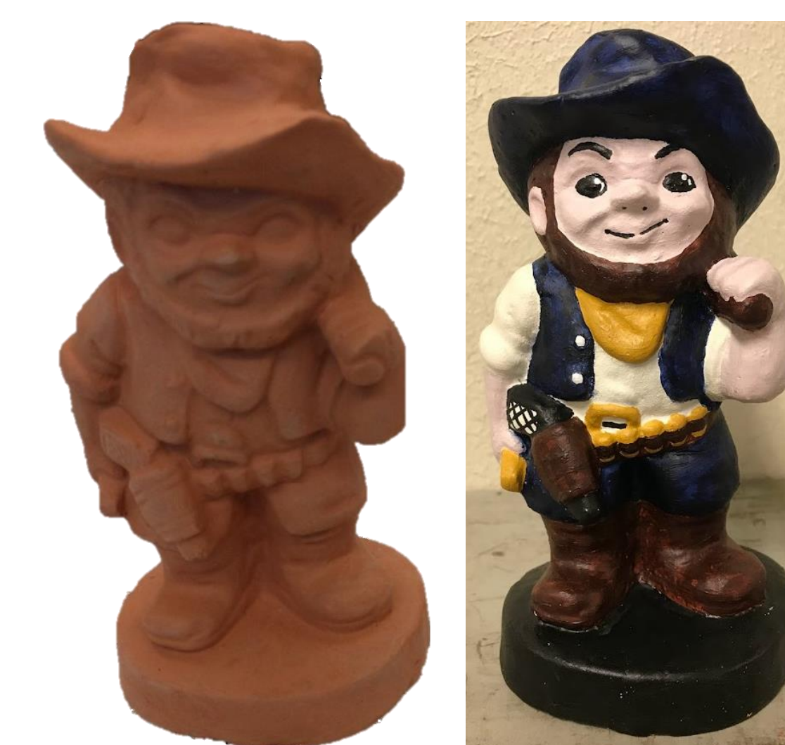
Figure 7: Image from a MET 352 team's final design presentation. The students made a mold around a statue of South Dakota Mines mascot, "Grubby". The students slip cast into the mold, fired the clay body (image on right), glazed the body, and then acrylic painted (image on the right) the ceramic body.
