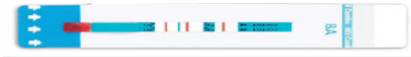
↑ SP ↑ CP ↑ LTA ↑ UTA ↑ CA SP = Sample Pad; CP = Conjugate Pad; LTA = Lower Test Area; UTA = Upper Test Area; CA = Control Area
