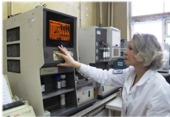
Gas Analyzer for infra-red absorption measurements. Definition range is from 0.001 to 2.0%.
