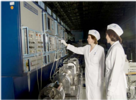
Non-destructive ultrasonic and eddy current inspection of final rods and tubes
